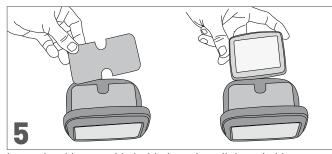
Insert the shims provided with the unit until the suitably shimmed navigator touches the clear surface of the case
