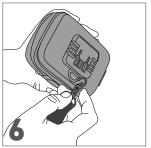
Hook the safety band to the case and fasten the Velcro closure on other end of the strap to the handlebar
